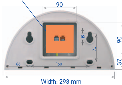
Space for RJ45 wall outlet
